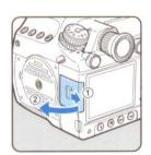
Insert the card all the way into the SD1 or SD2 slot with the SD Memory Card label facing toward the monitor.
