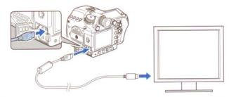
Connect the other end of the video cable or HDMI cable to the video IN jack or HDMI IN jack on the AV equipment, and then turn on the camera and AV equipment.
